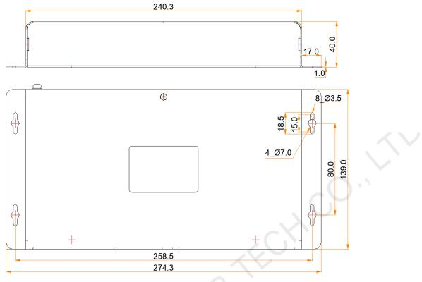
Tolerance: ±0.3 Unit: mm
