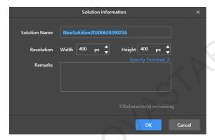
Figure 2-7 Solution information for an ultra-long screen
