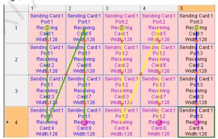
If you want to set receiving cards to blank, you can only set the receiving cards at both ends to blank, as shown in Figure 3-8 and Figure 3-9.
