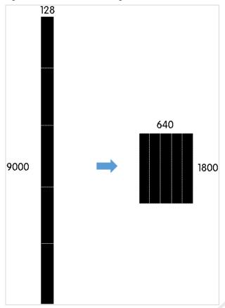
When you set the connection of receiving cards and an Ethernet port loads two rows/columns or more, the connection must follow the shape of the letter Z, as shown in Figure 3-6 and Figure 3-7.
