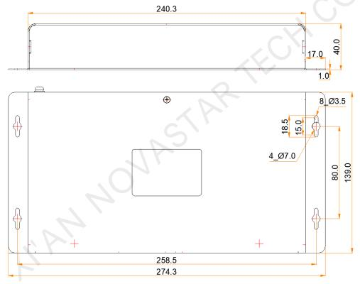
Tolerance: ±0.3 Unit: mm
